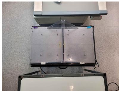
3. The detector on the **left** side of the calibration cage must be connected to the tethering cable with the matching purple tape, as shown below.
